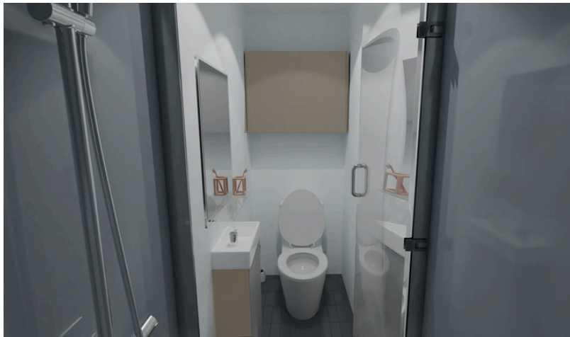
900 x 900 shower lined with 2 mm acrylic sheets for easy cleaning and to have the most of the usable space available for showering.
